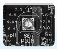
Press the "Read Set" key to adjust the setting. Setting is done in steps of 0.2 pH.
