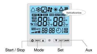
3. After a few seconds the display shows ROOM and a temperature. This is the temperature of the air surrounding the heat pump.
